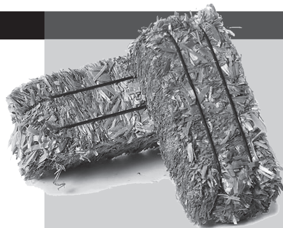
Those are not granola bars - they are bales of straw - used for home insulation!
